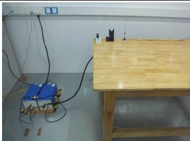
Conducted Emissions Test Setup View 1
