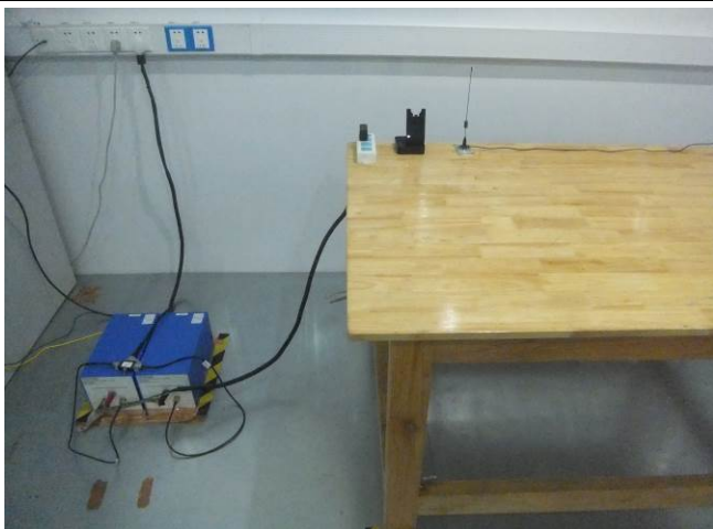
Radiated Spurious Emissions Test Setup Above 1GHz
