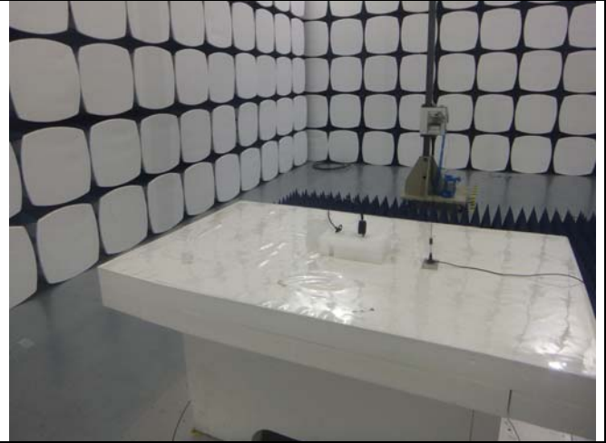
Radiated Spurious Emissions Test Setup Above 1GHz
