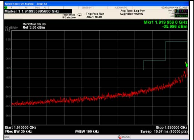
Out of band emission - 1915-1920 MHz High Channel
