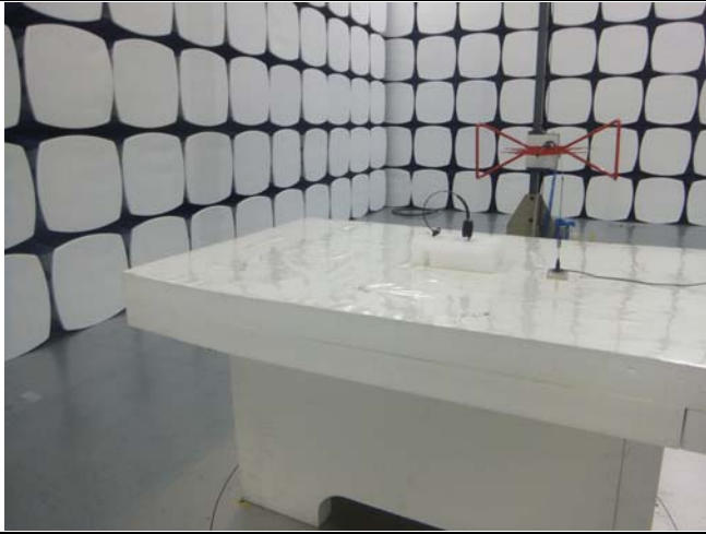
Radiated Spurious Emissions Test Setup Below 1GHz
