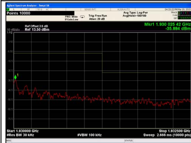
Out of band emission - 1930-1935 MHz Low Channel
