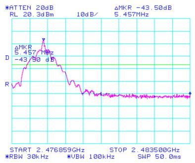
\* Above measured delta value is displayed at band edge point from lowest and highest frequency
