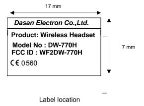
The label shown above shall be permanently affixed at a conspicuous location on the device and be readily visible to the user at the time purchase. The label is affixed with permanent adhesive to the enclosure and can not be readily detachable.
