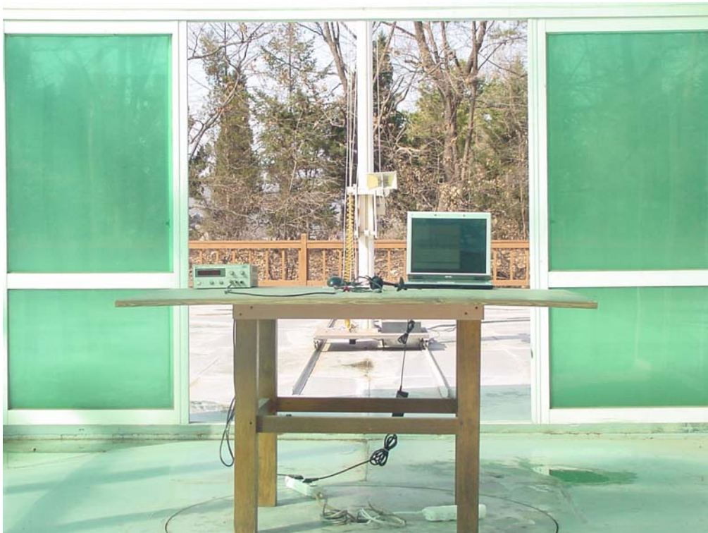
Radiated RF measurement (Above 1 GHz)
