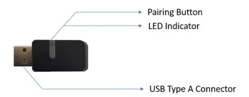
The BT-200 dongle is Bluetooth host device. So, Bluetooth headset can be paired with it. To make pairing, press the pairing button for a while. When it is on pairing mode, blue LED is blinking. If pairing is success, the blue LED stops blinking and turns on.
