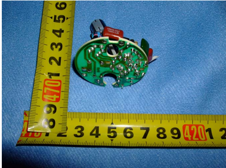
FE225 3016 & FE225 3015 Main Board - Soldered Side View
