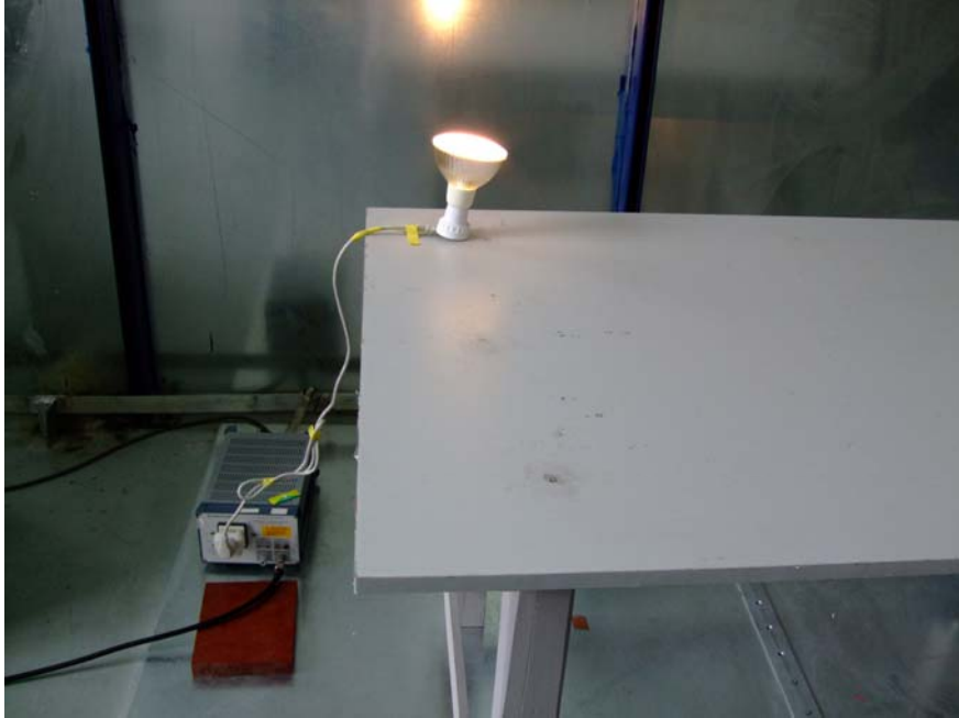
Conducted Emission Test Set-up - Front View
