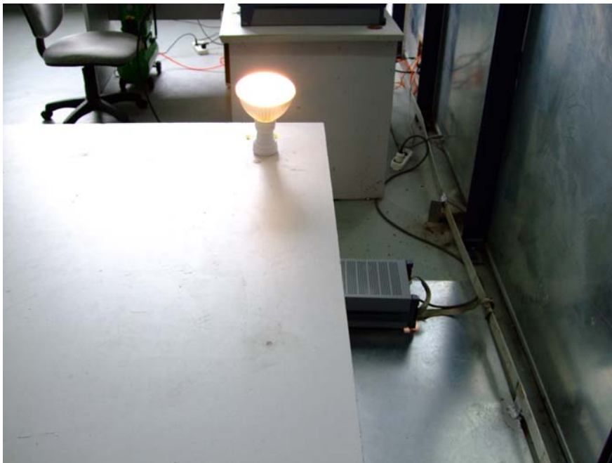
Conducted Emission Test Set-up - Side View
