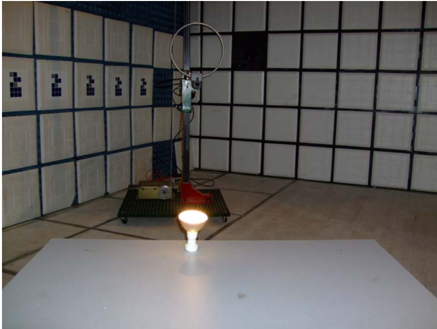
Radiated Emission Test Set-Up - Front View
