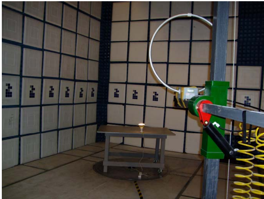
Radiated Emission Test Set-Up - Back View
