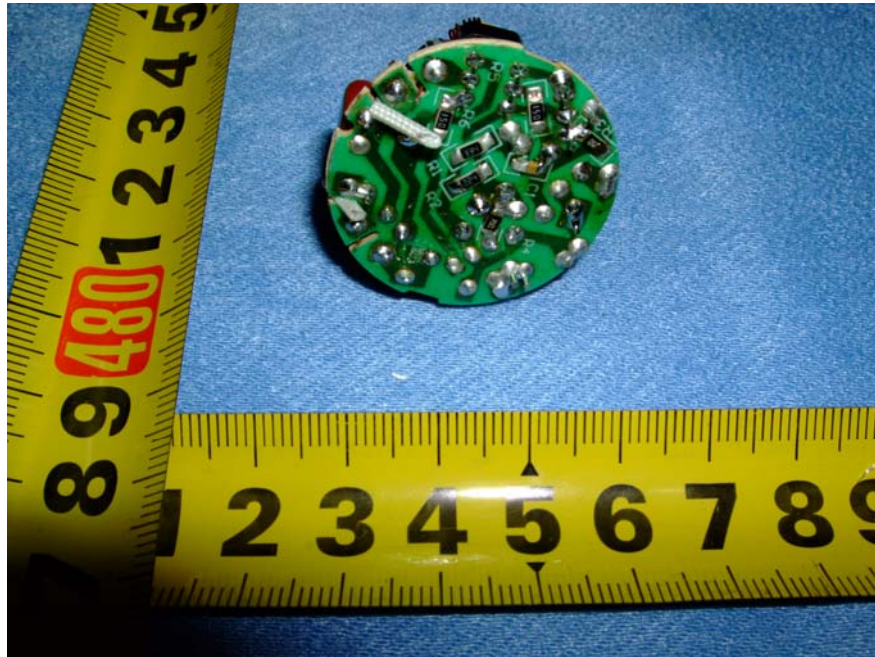
FE172 13S Main Board - Soldered Side View
