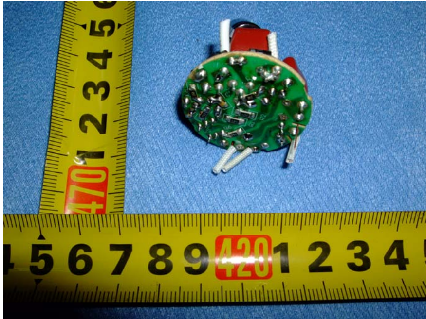
FE172 7S Main Board - Soldered Side View
