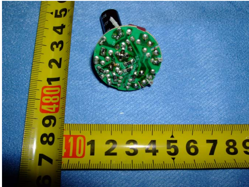
FE172 9S Main Board - Soldered Side View
