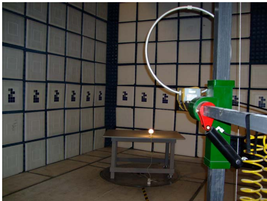
Radiated Emission Test Set-Up - Back View
