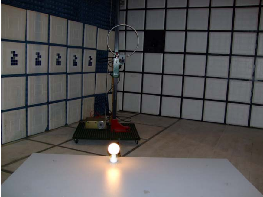
Radiated Emission Test Set-Up - Front View
