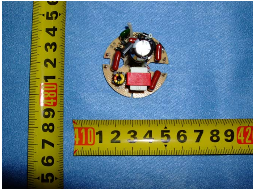
FE117 11W & FE117 9W Main Board - Component Side View
