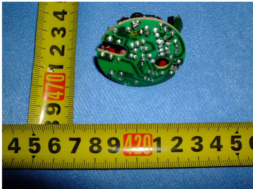
FE117 15W & FE117 14W Main Board - Soldered Side View
