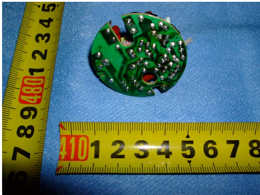
FE117 11W & FE117 9W Main Board - Soldered Side View
