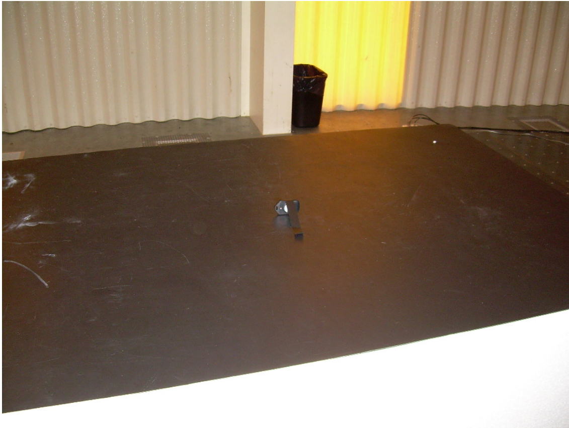
Photograph 2 - View Radiated Disturbance On-Edge Placement
