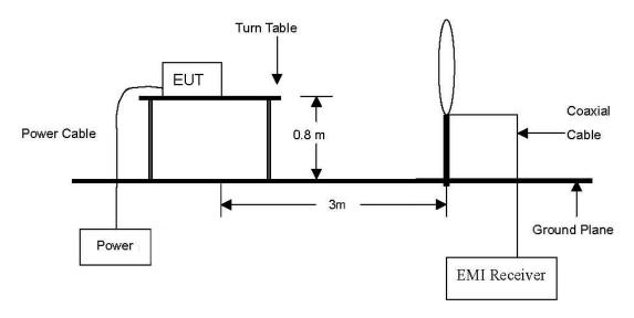
The diagram below shows the test setup that is utilized to make the measurements for emission from 30  $\,\text{Mz}$  to 1  $\,\text{GHz}$  Emissions.
