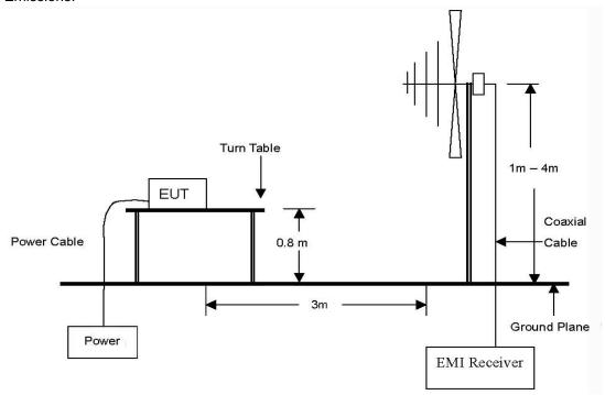
The diagram below shows the test setup that is utilized to make the measurements for emission from 1  $\times$  to 26.5  $\times$  Emissions.
