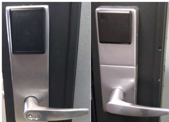
Inside escutcheon (antenna location)
