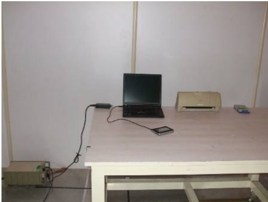
Conducted Emission Test Setup
