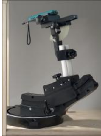
Fig. 15-4 Device Holder for Transmitters
