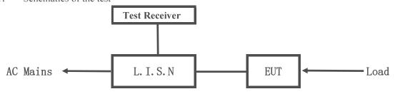
EUT: Equipment Under Test
