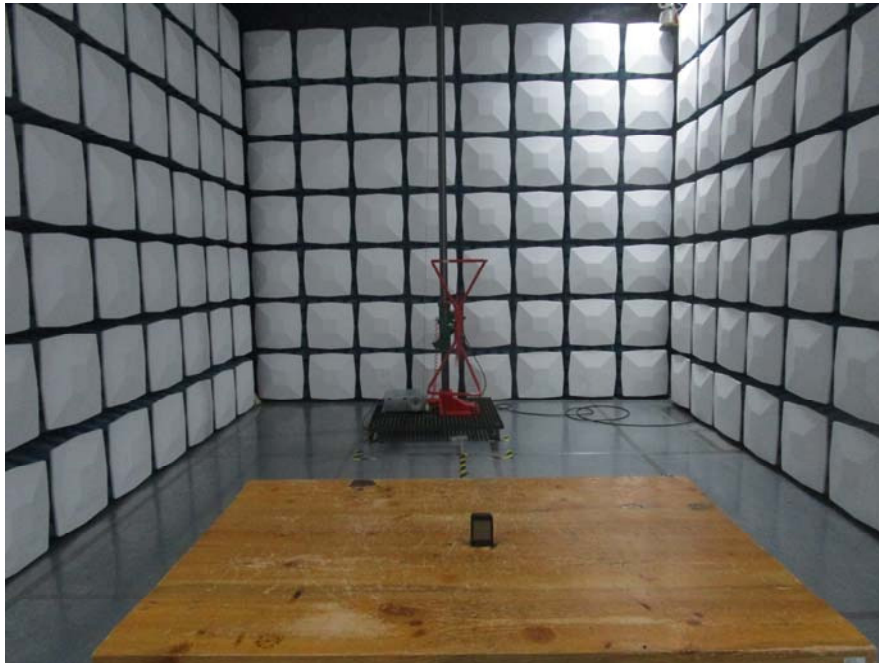
Radiated Emission View (Below 1GHz)
