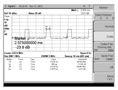
Duty Cycle Correction Factor= 20\*log [(18 x0.45ms) / 60.62ms]=-17.48dB
