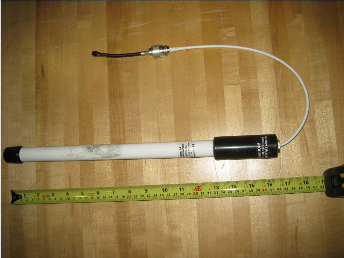
EUT – Antenna as as per 15.204(b)
