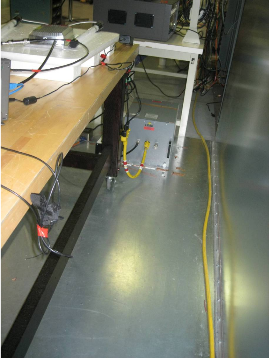
Power Line Conducted Emissions Photo 2
