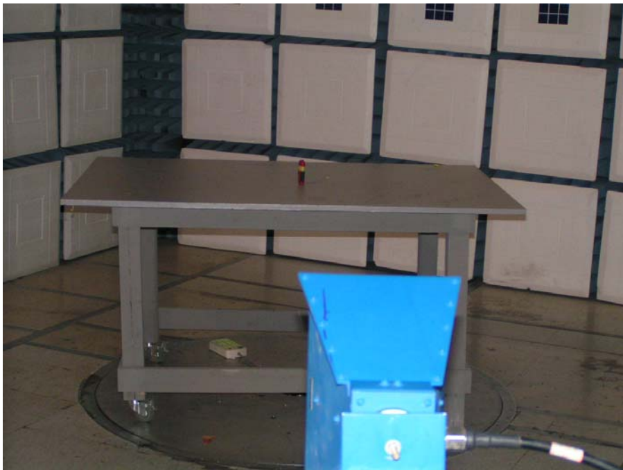
Field Strength Emissions Test Set-up - Lying mode
