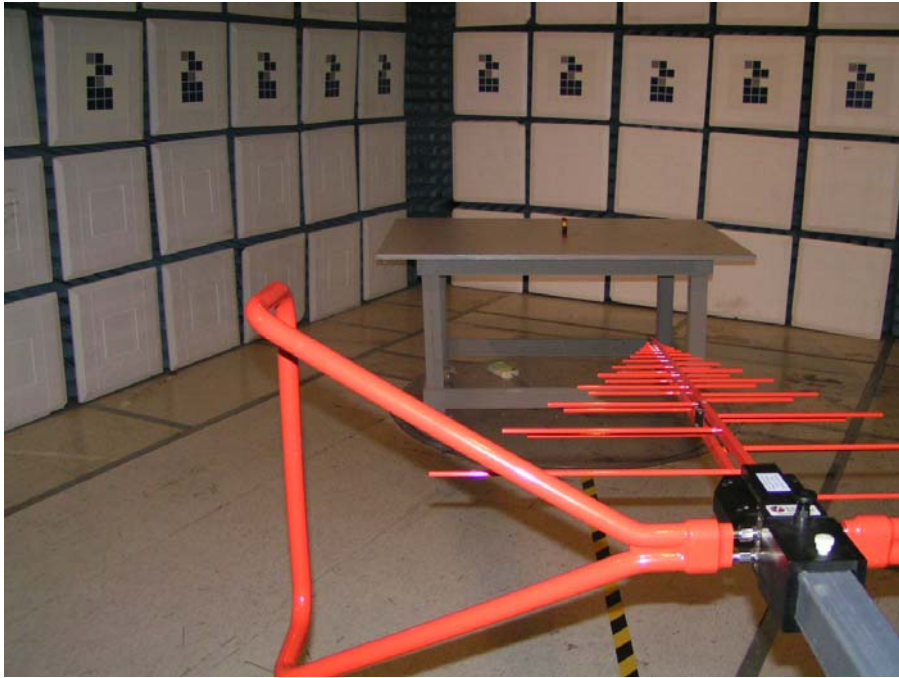
Field Strength Emissions Test Set-up - Stand mode
