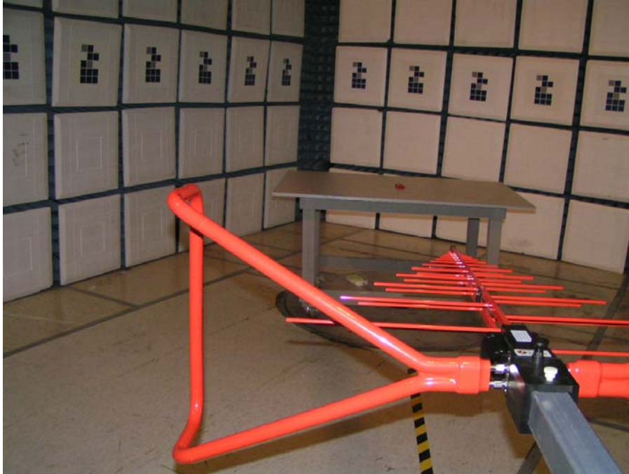
Field Strength Emissions Test Set-up (Below 1GHz)
