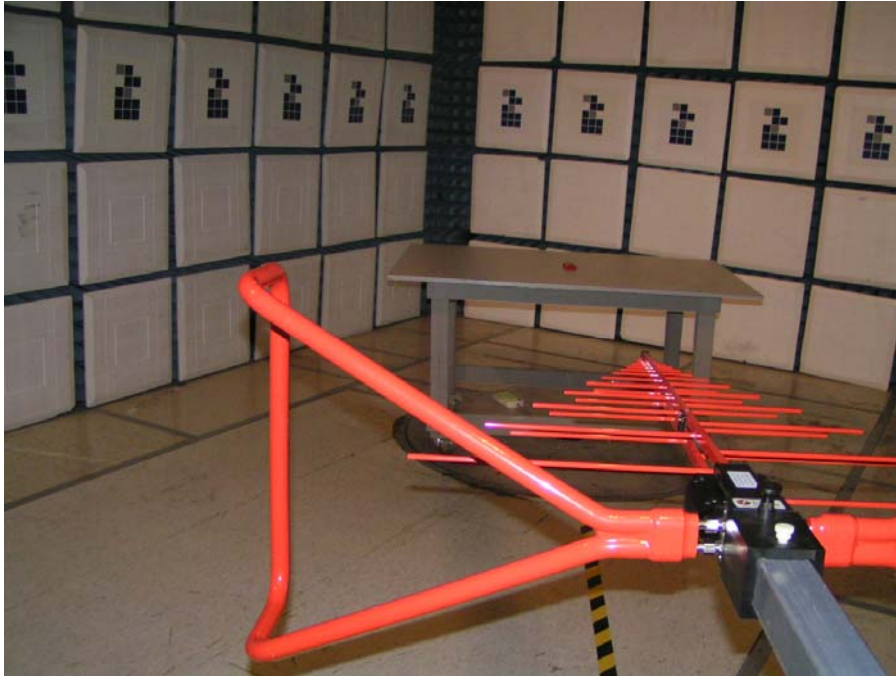
Field Strength Emissions Test Set-up - Lying mode
