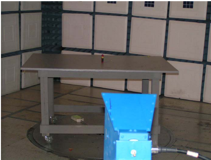
Field Strength Emissions Test Set-up - Stand mode
