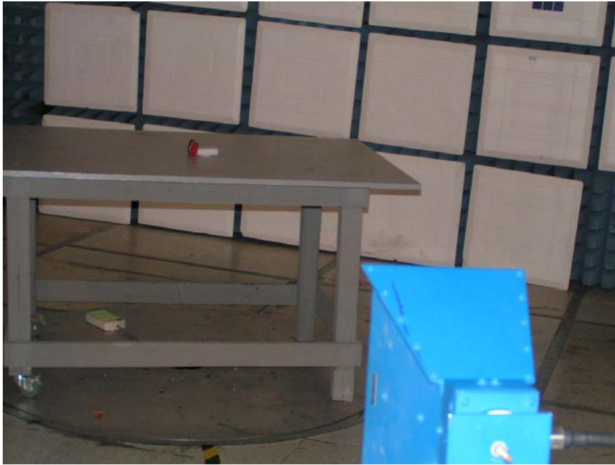
Field Strength Emissions Test Set-up - Side mode
