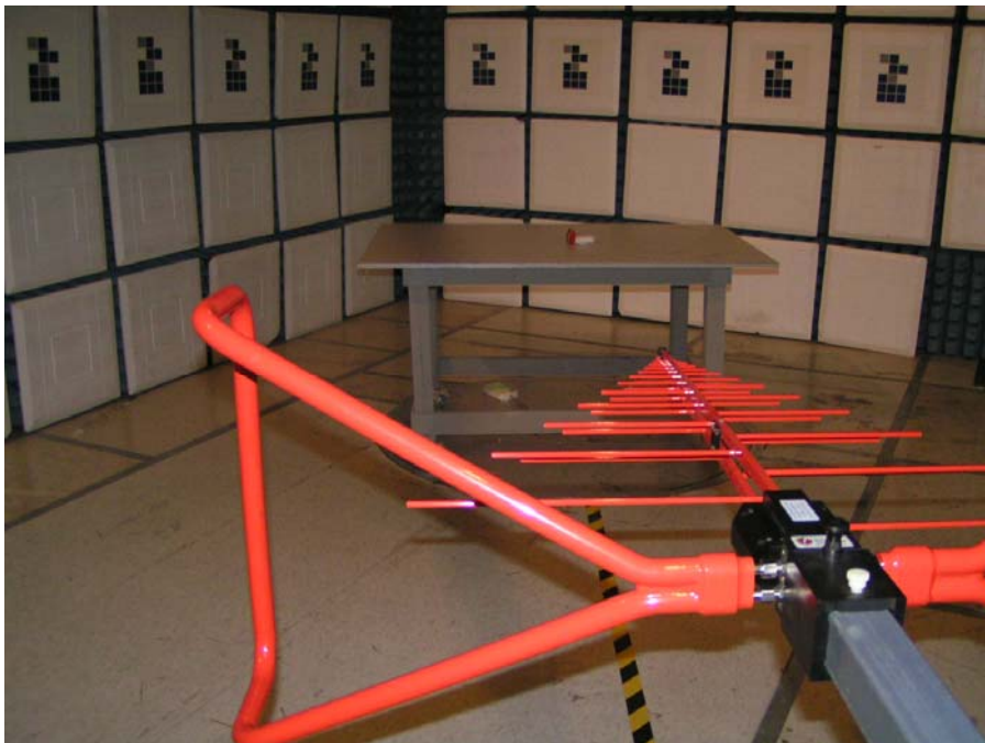
Field Strength Emissions Test Set-up - Side mode
