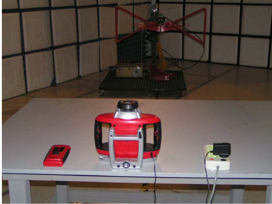
Radiated Emission Test Set-Up - Front View
