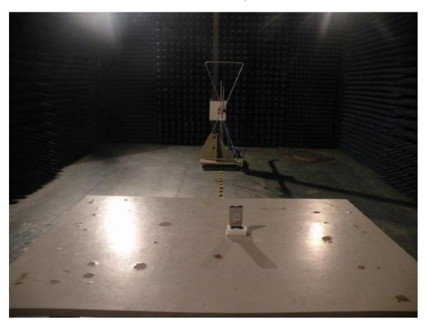
Radiated Emission Test Setup in Chamber
