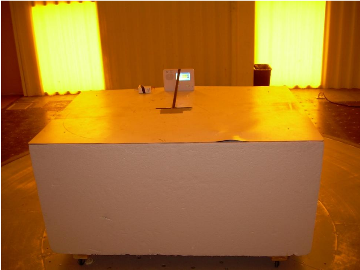
Photograph 1 – Front View Radiated Disturbance Worst Case Configuration
