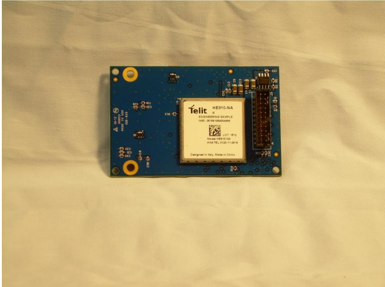
Photograph 17 – Back View of the 2G/3G Cell Modem
