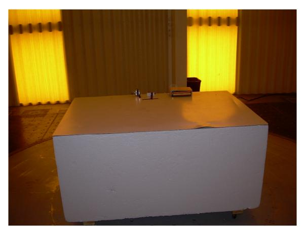
Front View Radiated Disturbance - Horizontal Configuration
