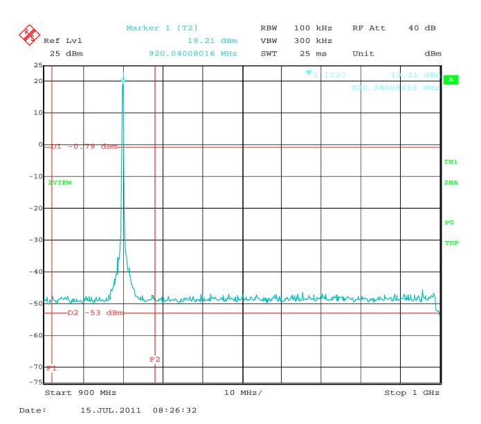
RF Antenna Conducted Test – High Channel – 900 MHz to 1 GHz
