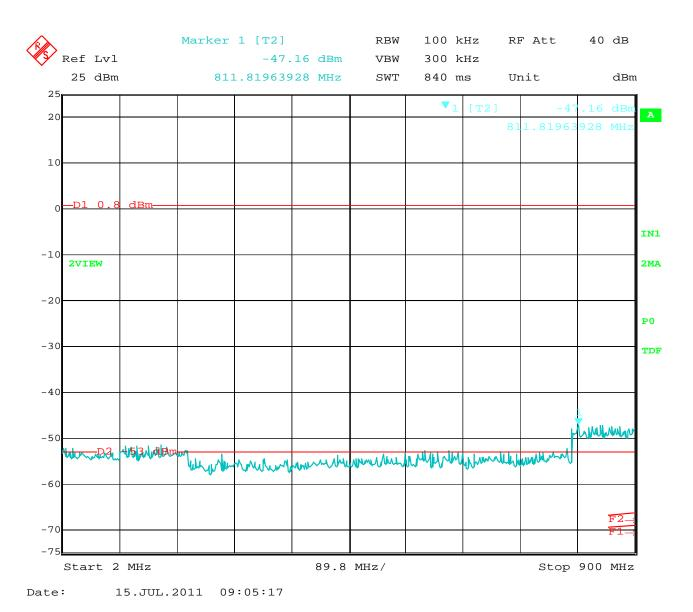
RF Antenna Conducted Test – Low Channel – 2 MHz to 900 MHz
