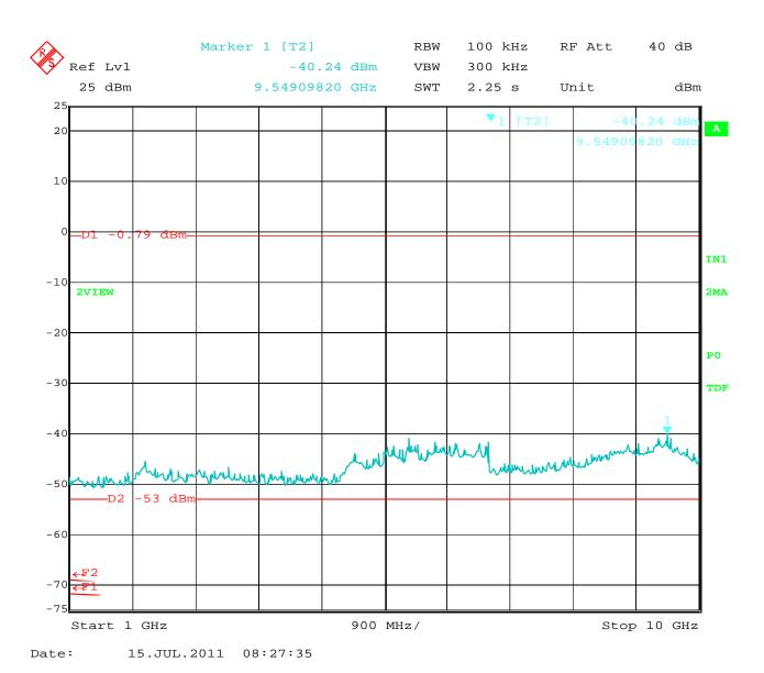
RF Antenna Conducted Test – High Channel – 1 GHz to 10 GHz
