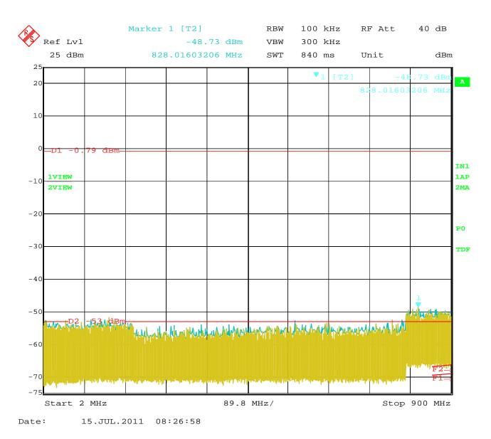
RF Antenna Conducted Test – High Channel – 2 MHz to 900 MHz
