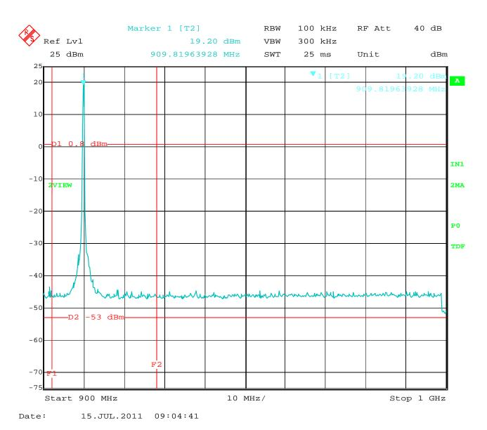
RF Antenna Conducted Test – Low Channel – 900 MHz to 1 GHz
