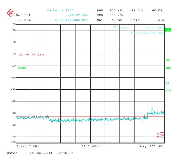
RF Antenna Conducted Test – Middle Channel – 2 MHz to 900 MHz
