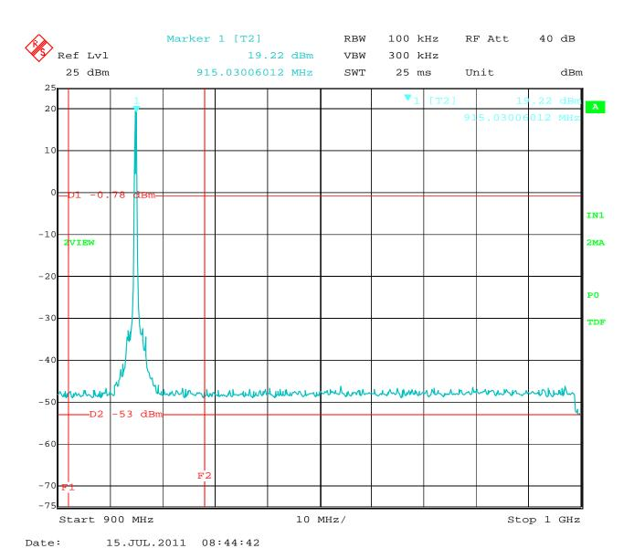
RF Antenna Conducted Test – Middle Channel – 900 MHz to 1 GHz
