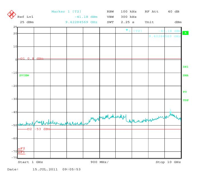
RF Antenna Conducted Test – Low Channel – 1 GHz to 10 GHz
