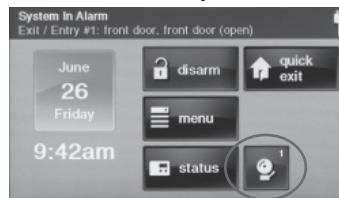
Security Screen with Alarm Memory Button
