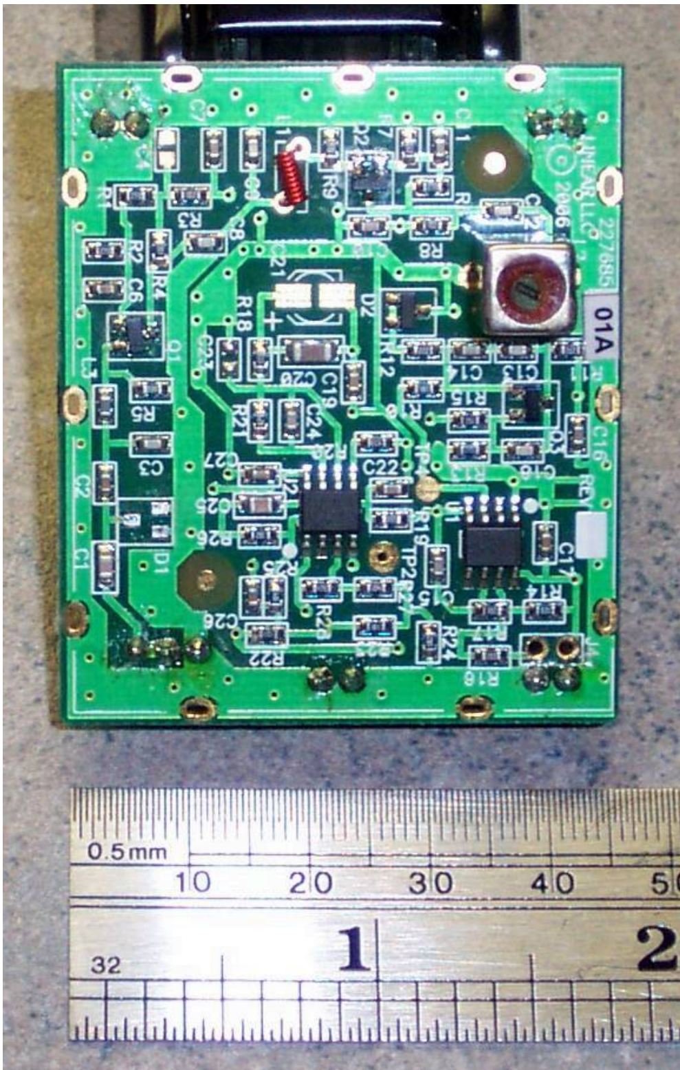
345 MHz Receiver Module. Shield Removed for clarity. Component Side View.
