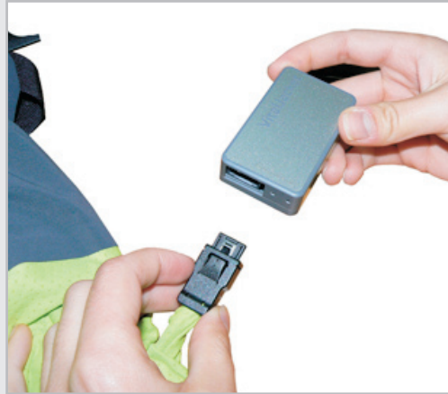
Fig. 12 – Connecting the electronic device to the T-Shirt plug.
