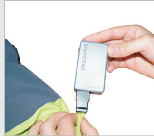
Fig. 13 – Storing the electronic device in the T-Shirt pocket.
