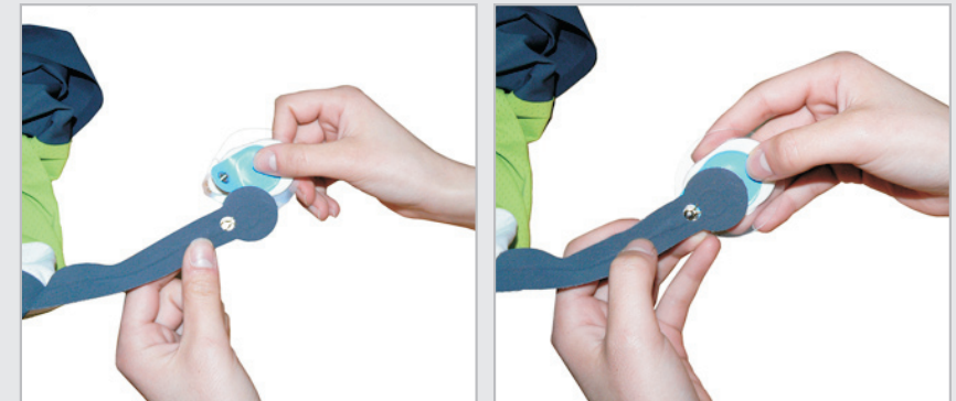
Fig. 7 – Connecting an electrode to a T-Shirt spring.
