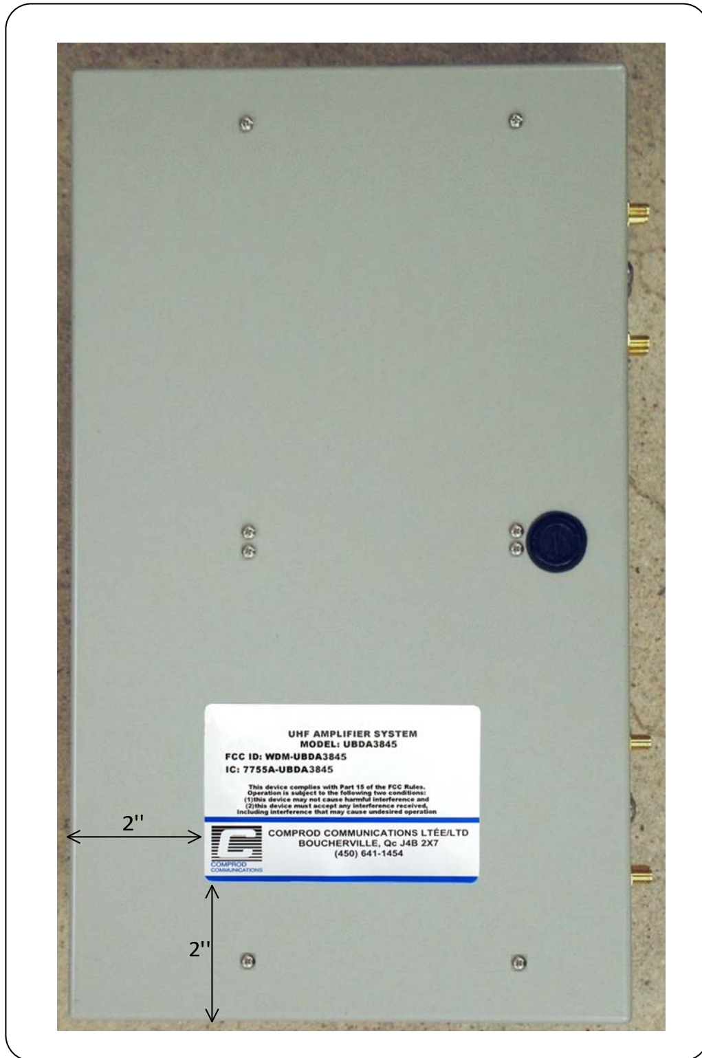
Figure 4: Label position on the BDA unit
