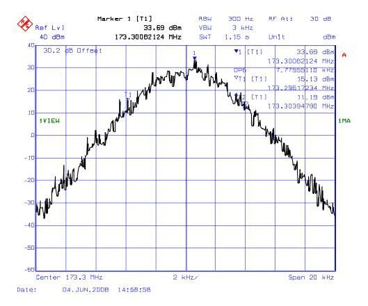
PLOT # 24(a): 99% Occupied Bandwidth – RF Input Signal
