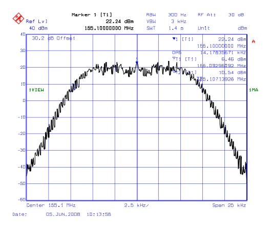
PLOT # 21(a): 99% Occupied Bandwidth – RF Input Signal Frequency: 161.9 MHz for 12.5 kHz Channel Spacing Modulation: FM modulation with 9600 b/s random data (F1D)
