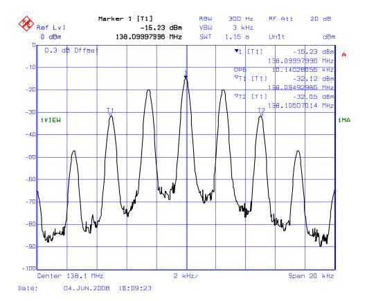
PLOT # 9(b): 99% Occupied Bandwidth – RF Output Signal Frequency: 138.1 MHz for 25 kHz Channel Spacing Modulation: FM modulation with 2.5 kHz Sinewave Signal (F3E)
