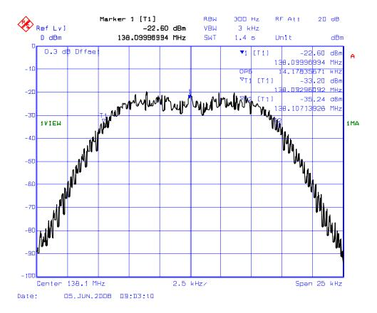
PLOT # 18(b): 99% Occupied Bandwidth - RF Output Signal Frequency: 138.1 MHz for 25 kHz Channel Spacing
