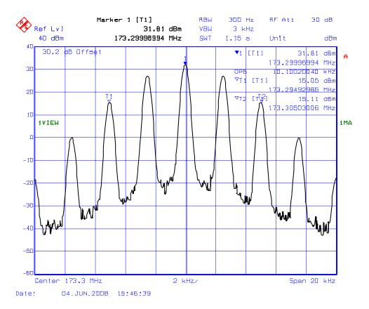
PLOT # 16(a): 99% Occupied Bandwidth – RF Input Signal Frequency: 173.3 MHz for 25 kHz Channel Spacing Modulation: FM modulation with 2.5 kHz Sinewave Signal (F3E)
