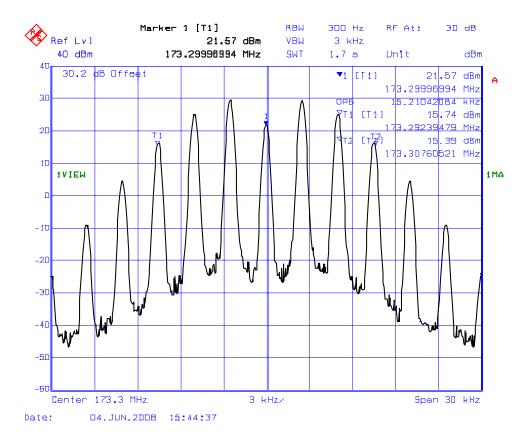
PLOT # 17(a): 99% Occupied Bandwidth – RF Input Signal Frequency: 138.1 MHz for 12.5 kHz Channel Spacing
