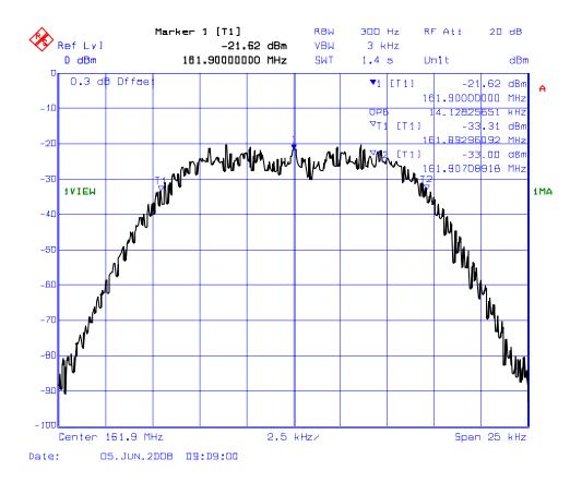
PLOT # 22(b): 99% Occupied Bandwidth - RF Output Signal Frequency: 161.9 MHz for 25 kHz Channel Spacing
