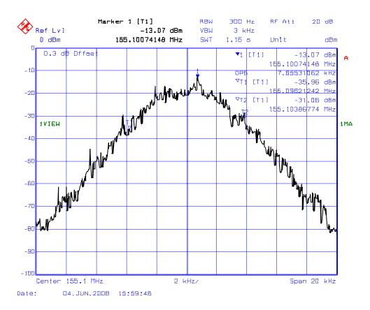
PLOT # 19(b): 99% Occupied Bandwidth – RF Output Signal Frequency: 155.1 MHz for 12.5 kHz Channel Spacing
