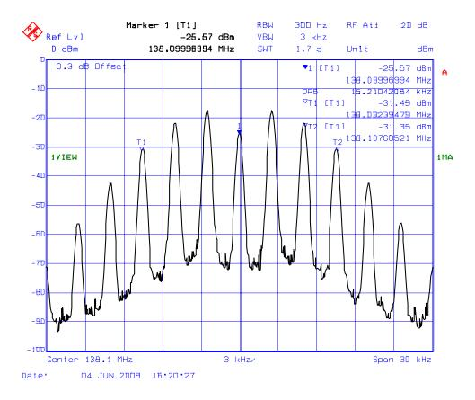
PLOT # 10(b): 99% Occupied Bandwidth - RF Output Signal Frequency: 138.1 MHz for 25 kHz Channel Spacing Modulation: FM modulation with 2.5 kHz Sinewave Signal (F3E)
