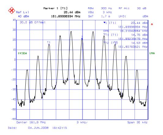
PLOT # 15(a): 99% Occupied Bandwidth – RF Input Signal Frequency: 173.3 MHz for 12.5 kHz Channel Spacing Modulation: FM modulation with 2.5 kHz Sinewave Signal (F3E)
