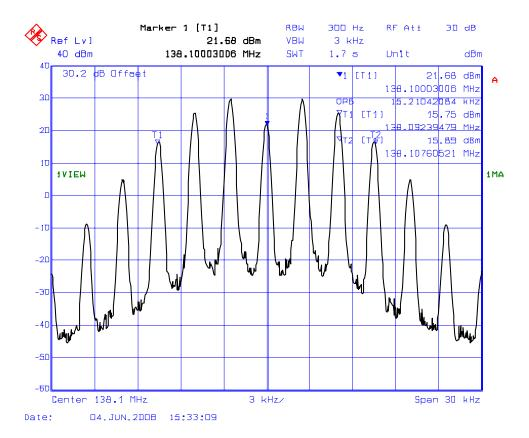
PLOT # 11(a): 99% Occupied Bandwidth - RF Input Signal Frequency: 155.1 MHz for 12.5 kHz Channel Spacing Modulation: FM modulation with 2.5 kHz Sinewave Signal (F3E)
