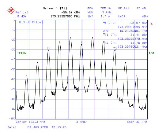
PLOT # 16(b): 99% Occupied Bandwidth – RF Output Signal Frequency: 173.3 MHz for 25 kHz Channel Spacing Modulation: FM modulation with 2.5 kHz Sinewave Signal (F3E)
