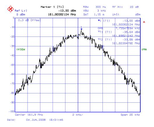
PLOT # 21(b): 99% Occupied Bandwidth – RF Output Signal Frequency: 161.9 MHz for 12.5 kHz Channel Spacing Modulation: FM modulation with 9600 b/s random data (F1D)
