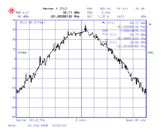
PLOT # 22(a): 99% Occupied Bandwidth – RF Input Signal Frequency: 161.9 MHz for 25 kHz Channel Spacing Modulation: FM modulation with 9600 b/s random data (F1D)
