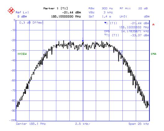
PLOT # 20(b): 99% Occupied Bandwidth – RF Output Signal Frequency: 155.1 MHz for 25 kHz Channel Spacing
