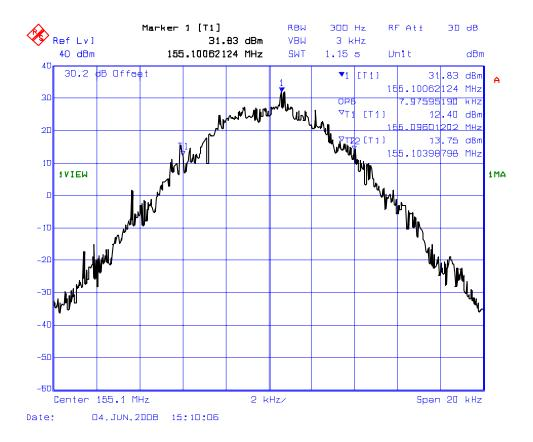
PLOT # 20(a): 99% Occupied Bandwidth – RF Input Signal
