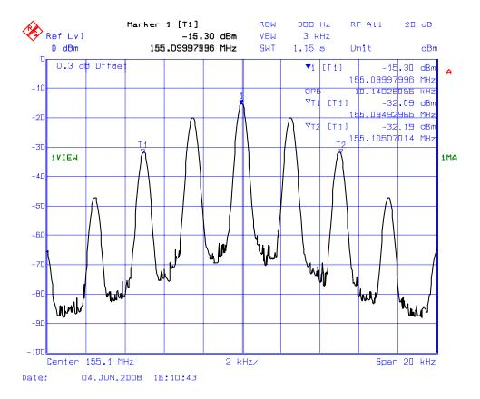
PLOT # 11(b): 99% Occupied Bandwidth – RF Output Signal Frequency: 155.1 MHz for 12.5 kHz Channel Spacing Modulation: FM modulation with 2.5 kHz Sinewave Signal (F3E)
