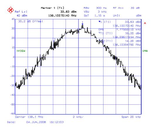
PLOT # 18(a): 99% Occupied Bandwidth – RF Input Signal
