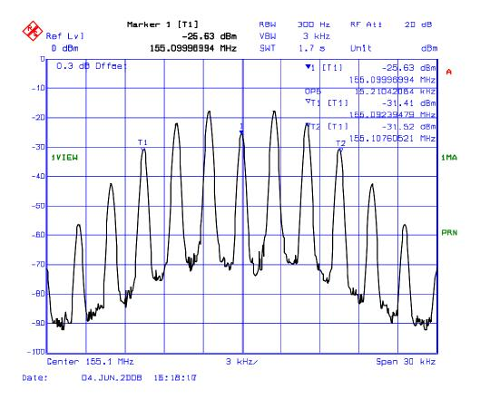
PLOT # 12(b): 99% Occupied Bandwidth – RF Output Signal Frequency: 155.1 MHz for 25 kHz Channel Spacing Modulation: FM modulation with 2.5 kHz Sinewave Signal (F3E)
