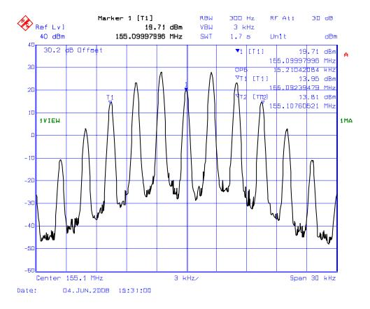
PLOT # 13(a): 99% Occupied Bandwidth – RF Input Signal Frequency: 161.9 MHz for 12.5 kHz Channel Spacing Modulation: FM modulation with 2.5 kHz Sinewave Signal (F3E)
