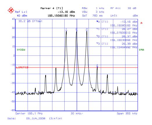
PLOT#: 7 Intermodulation with 3 RF signal inputs/outputs Fc= 161.9 MHz, Fc+25 kHz & Fc-25 kHz, RF Input levels = -61.8 dBm
