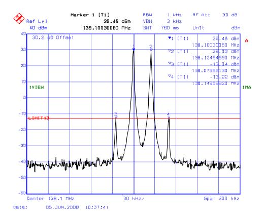
PLOT#: 2 Intermodulation with 2 RF signal inputs/outputs Fc= 155.1 MHz, Fc+25 kHz, RF Input levels = -15.3 dBm
