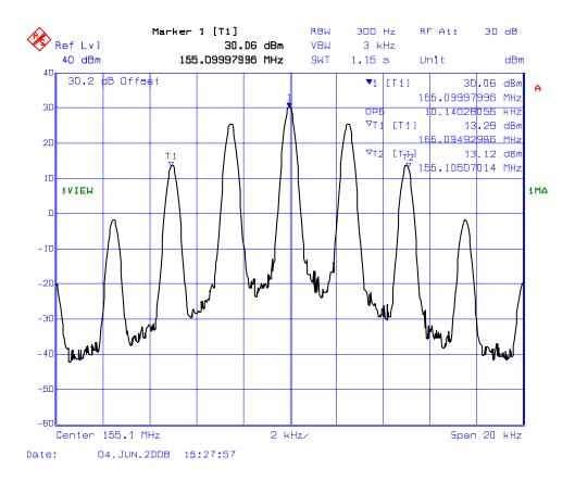
PLOT # 12(a): 99% Occupied Bandwidth – RF Input Signal Frequency: 155.1 MHz for 25 kHz Channel Spacing Modulation: FM modulation with 2.5 kHz Sinewave Signal (F3E)
