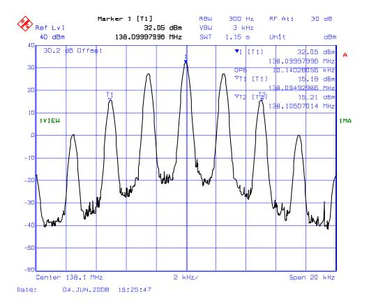
PLOT # 10(a): 99% Occupied Bandwidth - RF Input Signal Frequency: 138.1 MHz for 25 kHz Channel Spacing Modulation: FM modulation with 2.5 kHz Sinewave Signal (F3E)
