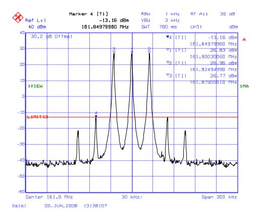
PLOT#: 8 Intermodulation with 3 RF signal inputs/outputs Fc= 173.3 MHz, Fc+25 kHz & Fc-25 kHz, RF Input levels = -61.8 dBm
