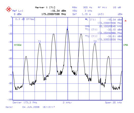
PLOT # 15(b): 99% Occupied Bandwidth – RF Output Signal Frequency: 173.3 MHz for 12.5 kHz Channel Spacing Modulation: FM modulation with 2.5 kHz Sinewave Signal (F3E)
