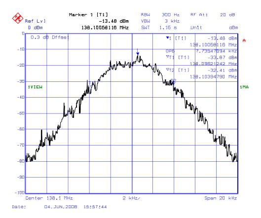
PLOT # 17(b): 99% Occupied Bandwidth - RF Output Signal Frequency: 138.1 MHz for 12.5 kHz Channel Spacing Modulation: FM modulation with 9600 b/s random data (F1D)
