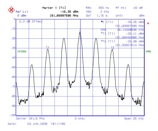
PLOT # 13(b): 99% Occupied Bandwidth – RF Output Signal Frequency: 161.9 MHz for 12.5 kHz Channel Spacing Modulation: FM modulation with 2.5 kHz Sinewave Signal (F3E)
