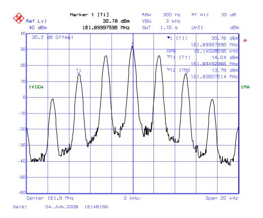
PLOT # 14(a): 99% Occupied Bandwidth – RF Input Signal Frequency: 161.9 MHz for 25 kHz Channel Spacing Modulation: FM modulation with 2.5 kHz Sinewave Signal (F3E)
