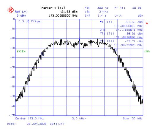
PLOT # 24(b): 99% Occupied Bandwidth – RF Output Signal Frequency: 173.3 MHz for 25 kHz Channel Spacing
