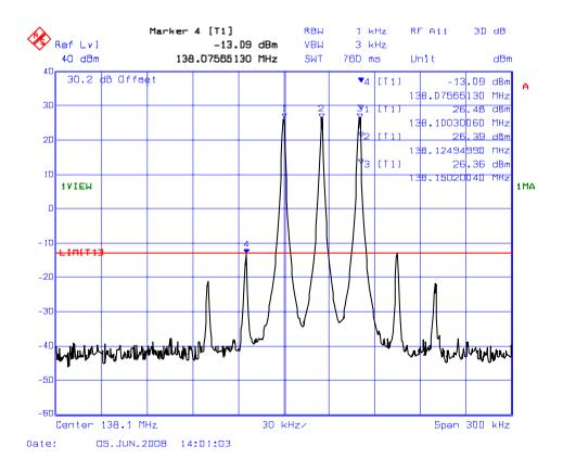
PLOT#: 6 Intermodulation with 3 RF signal inputs/outputs Fc= 155.1 MHz, Fc+25 kHz & Fc-25 kHz, RF Input levels = -61.7 dBm
