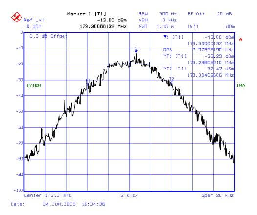
PLOT # 23(b): 99% Occupied Bandwidth – RF Output Signal Frequency: 173.3 MHz for 12.5 kHz Channel Spacing Modulation: FM modulation with 9600 b/s random data (F1D)
