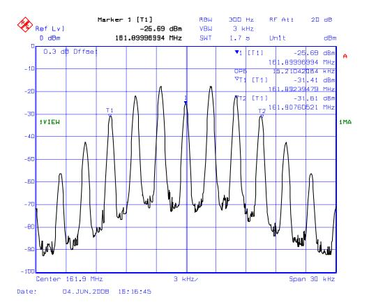
PLOT # 14(b): 99% Occupied Bandwidth – RF Output Signal Frequency: 161.9 MHz for 25 kHz Channel Spacing Modulation: FM modulation with 2.5 kHz Sinewave Signal (F3E)
