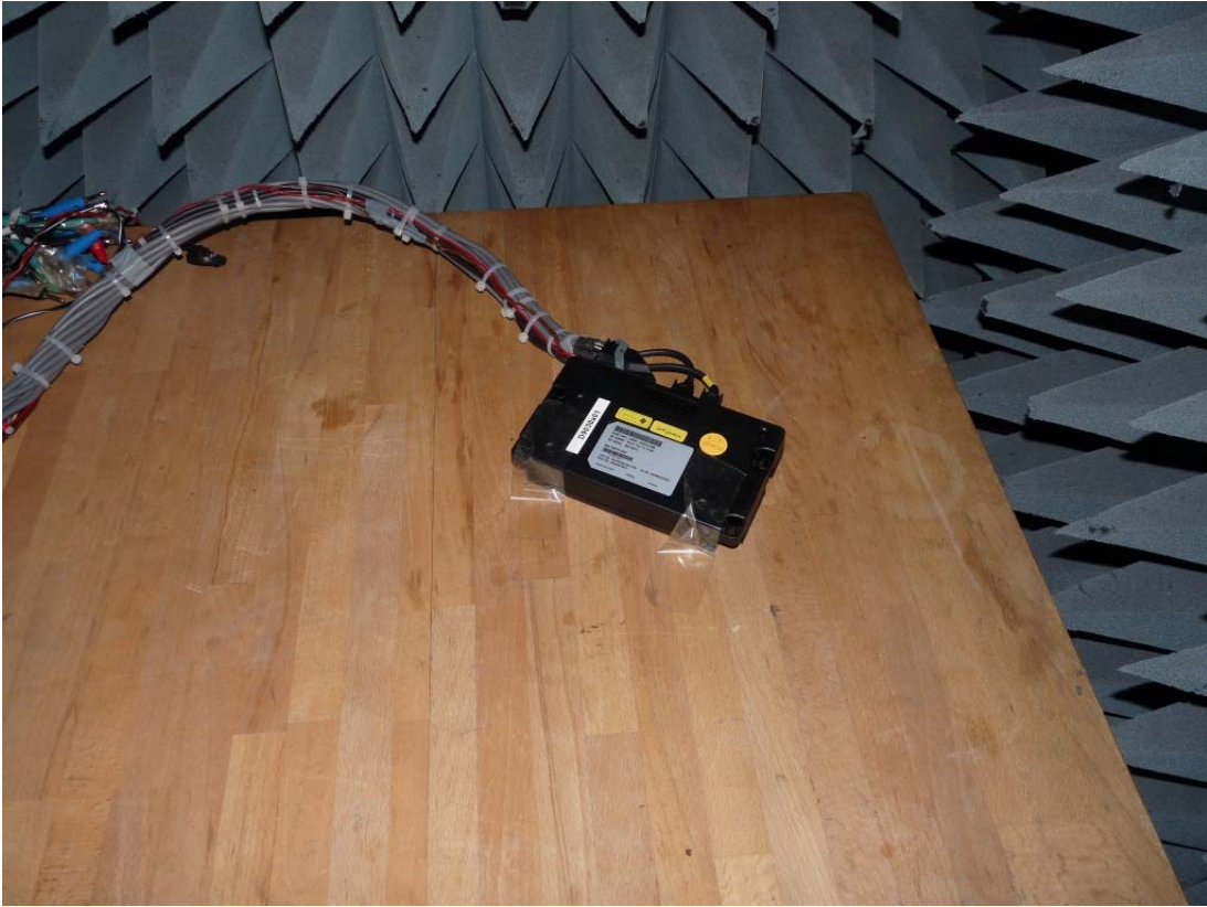
Photo 1: Setup for radiated measurements below 30 MHz
