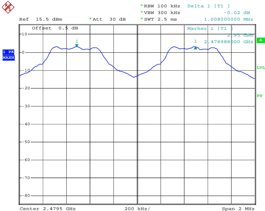
TOKWA channel separation high channel
