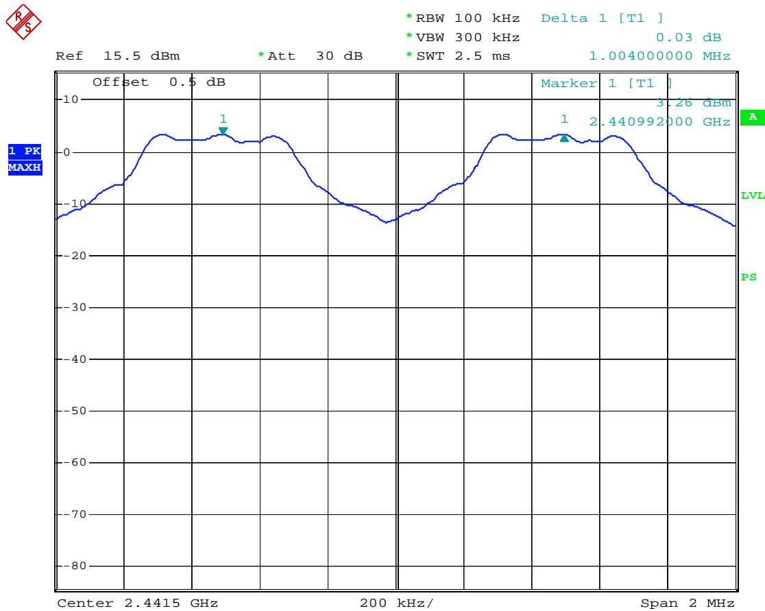
TOKWA channel separation middle channel
