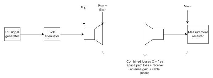
The signal level at the measurement receiver,  $M_{REF}$ , is recorded for each of the frequencies under test. Given that the transmit antenna is calibrated with a known gain  $G_{REF}$ , the following expression holds true:
