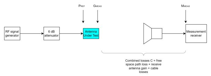
The peak received signal level at the measurement receiver is identified and noted as  $\mathbf{M}_{\text{MEAS}}$ .
