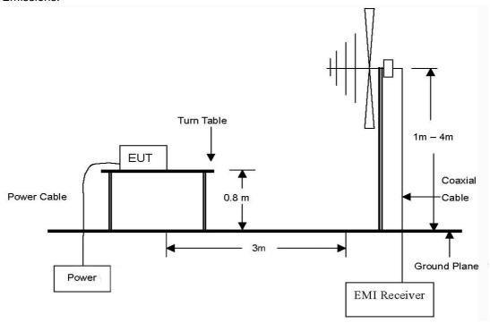
The diagram below shows the test setup that is utilized to make the measurements for emission .The spurious emissions were investigated form 1  $\mbox{GHz}$  to the 10th harmonic of the highest fundamental frequency or 40  $\mbox{GHz}$ , whichever is lower.
