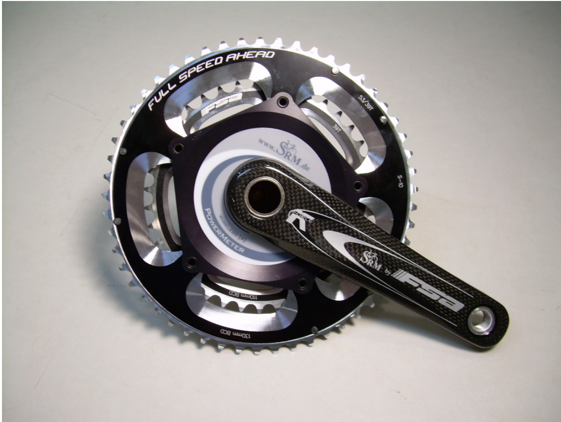
Photograph 5 - Back View of the PowerMeter6
