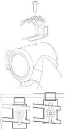
To mount the sensor magnet, remove the cable guide bolt and the cable guide below the bottom bracket.
