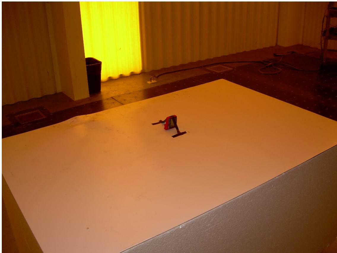
Radiated Set-Up - Horizontal Configuration
