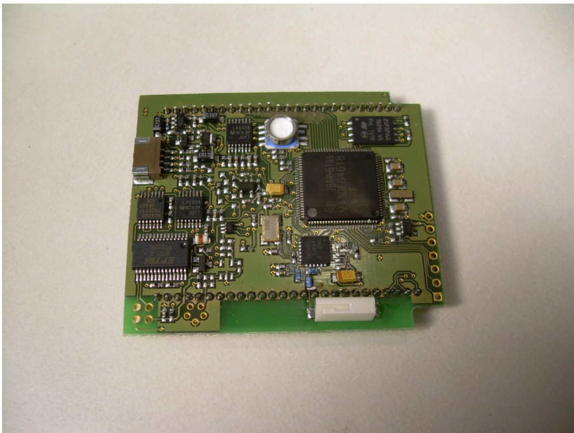
View of the Component Side of the PowerControl6 PCB
