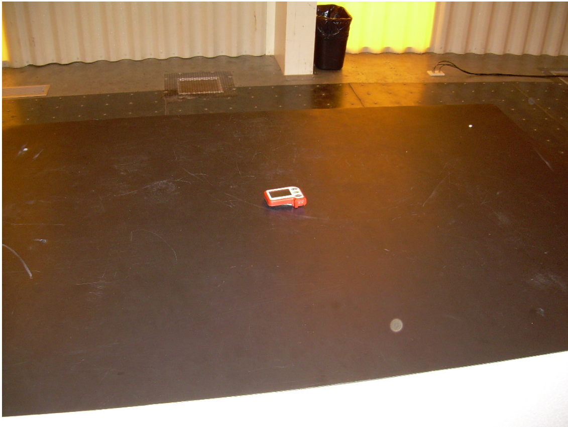
Photograph 1 - View Radiated Disturbance - Flat Placement - Worst Case Configuration
