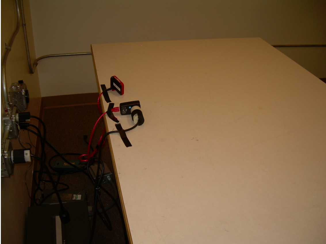
Photograph 6 - Back View Conducted Disturbance Worst Case Configuration
