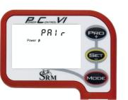
Hold **PP** for about 3 seconds to enter Sensor Pairing mode. Press **Press** once quickly to select the device you want to pair and press **PP** once quickly to tell the PC VI to start searching.
