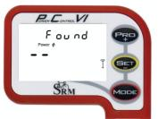
If a Sensor is found, the PC VI will show "Found" in the Top line, alternating with the Sensor's Serial number.
