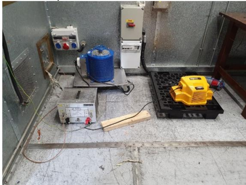
Photograph No.2 Setup for conducted emission measurements
