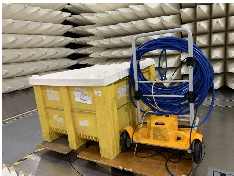
Photograph 7.2.2 Setup for radiated emission measurements, EUT cabling
