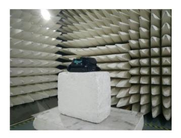
Photograph No.5 Setup for 20 dB bandwidth measurements
