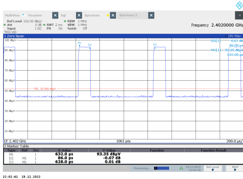
Plot 7.3.19 Transmission pulse period and duration
