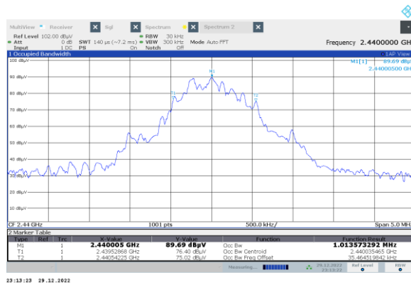
Plot 7.1.4 99% bandwidth test result at mid frequency
