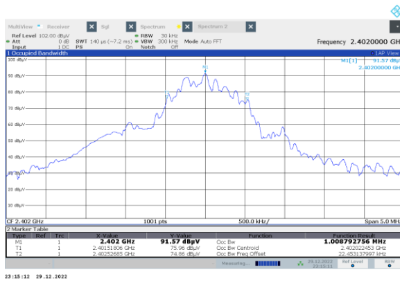
Plot 7.1.2 99% bandwidth test result at low frequency
