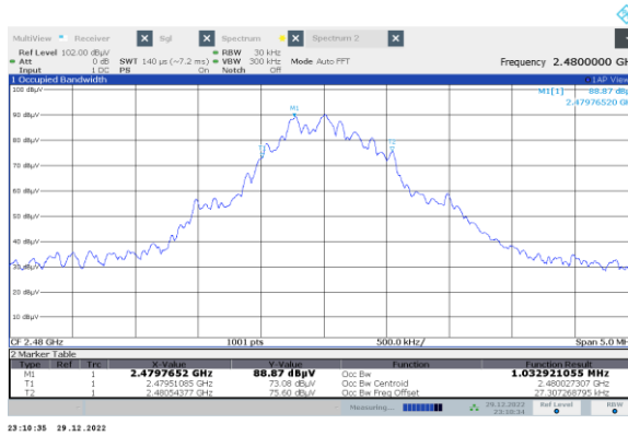
Plot 7.1.6 99% bandwidth test result at high frequency
