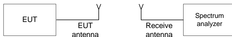
Figure 7.1.1 6 dB bandwidth test setup
