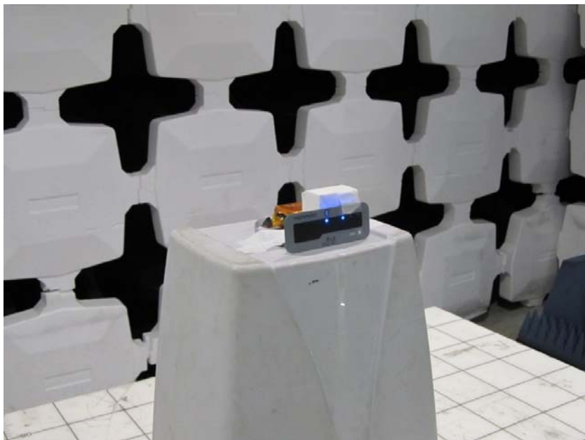
Photo 6. Radiated emissions test setup.
