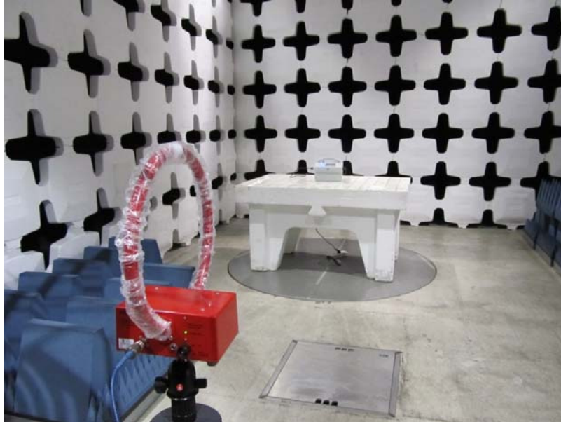
Photo 1.. Radiated emissions test setup with Loop antenna.
