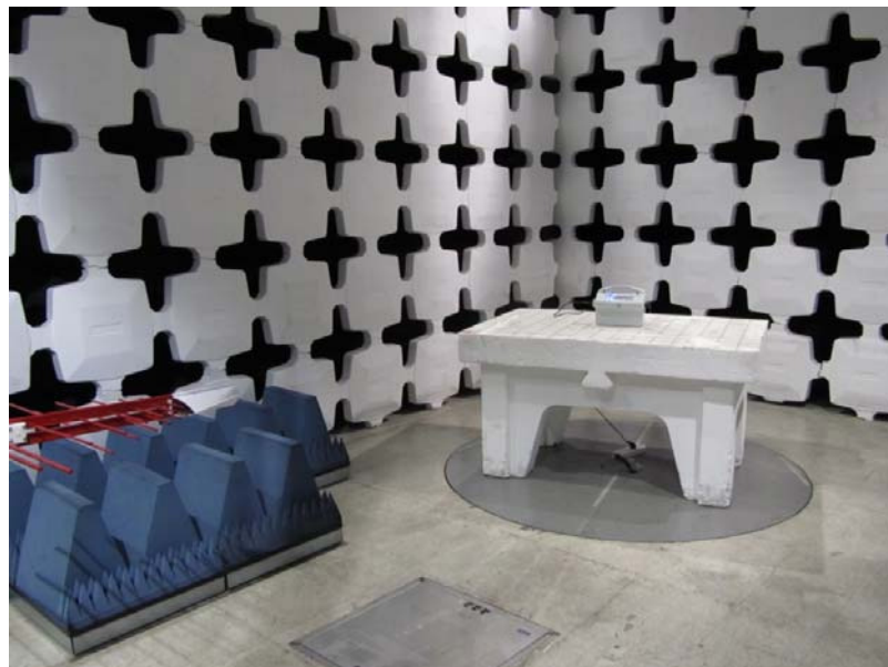
Photo 2. Radiated emissions test setup with Biconilog antenna.
