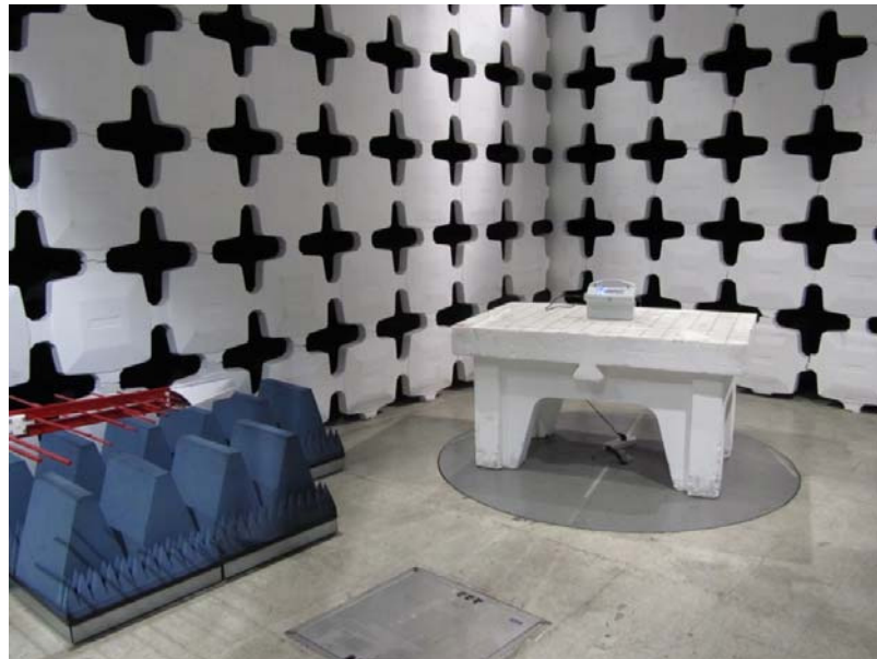
Photo 2. Radiated emissions test setup with Biconilog antenna.
