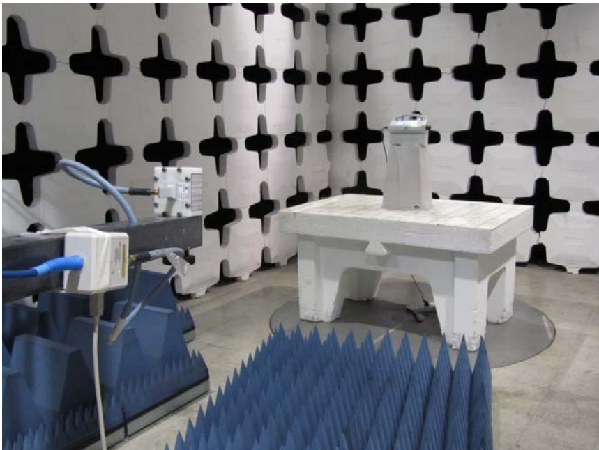
Photo 4. Radiated emissions test setup with Horn antenna in 18-25GHz.
