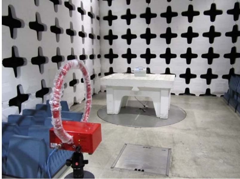
Photo 1.. Radiated emissions test setup with Loop antenna.
